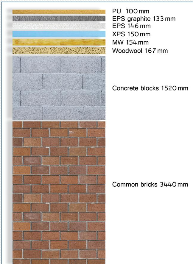
Figure 2: Thickness of different insulation and other materials at equal R-values
